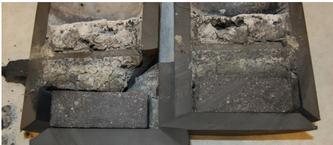
Figure 11. Cross-section of crucible after Test 10 with Olibar as bedding material.
