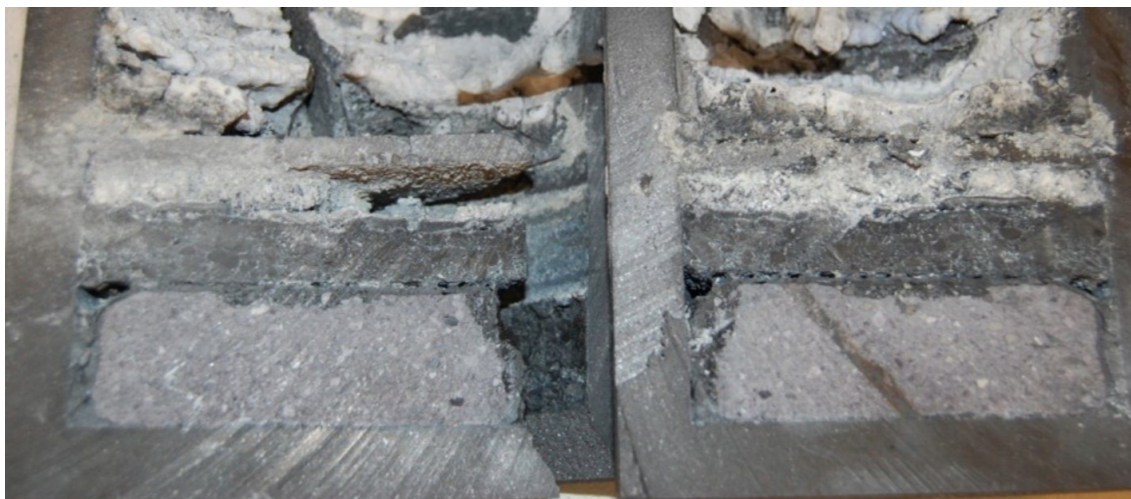
Figure 10. Cross-section of crucible after Test 9 with \text{AlF}_3 and ramming paste as bedding material.
