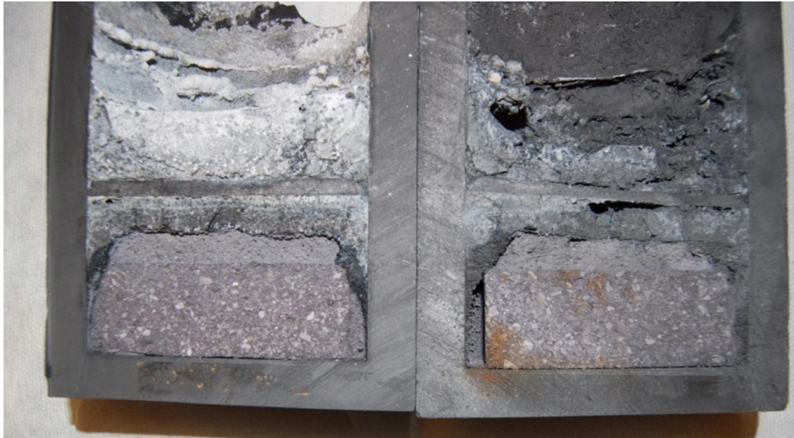
Figure 15. Comparison of parallel Test 4 (right) and Test 12 (left) Alubar 1100 as bedding material.
