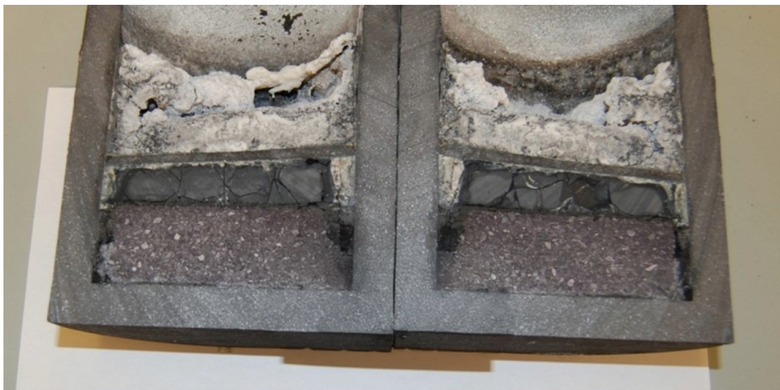
Figure 7. Cross-section of crucible after Test 6 with spent refractory brick as bedding material.
