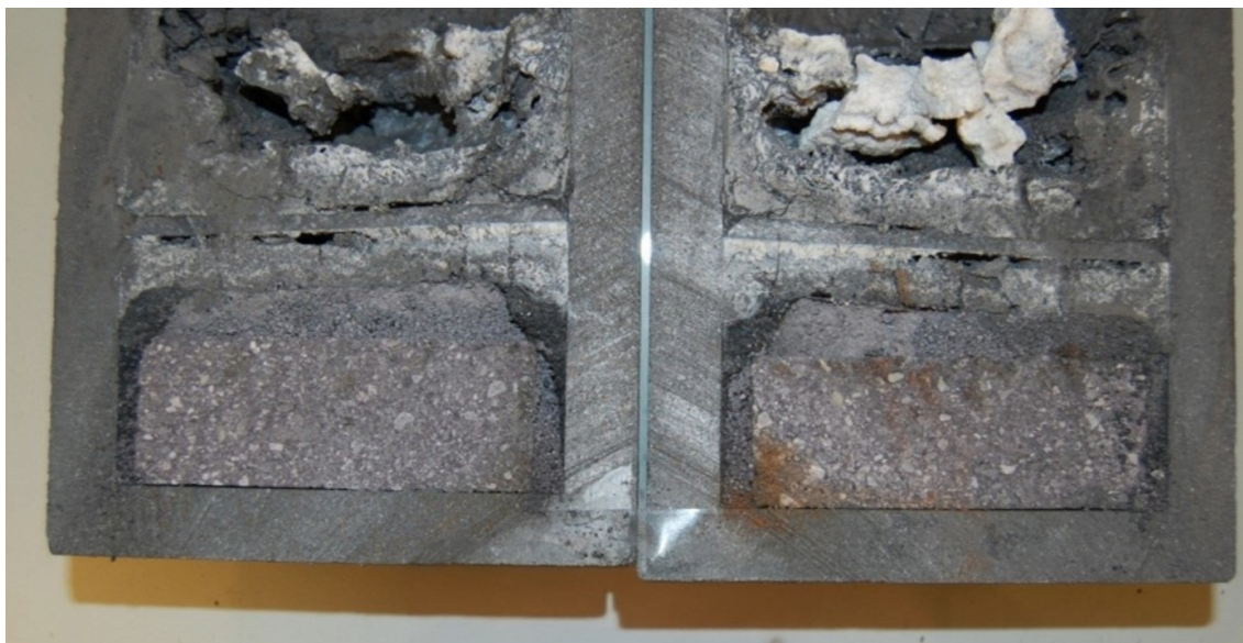
Figure 5. Cross-section of crucible after Test 4 with Alubar 1100 as bedding material.
