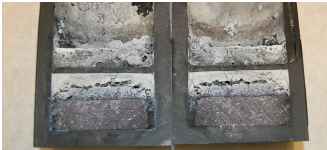
Figure 12. Cross-section of crucible after Test 11 with Al 2 O 3 as bedding material.
