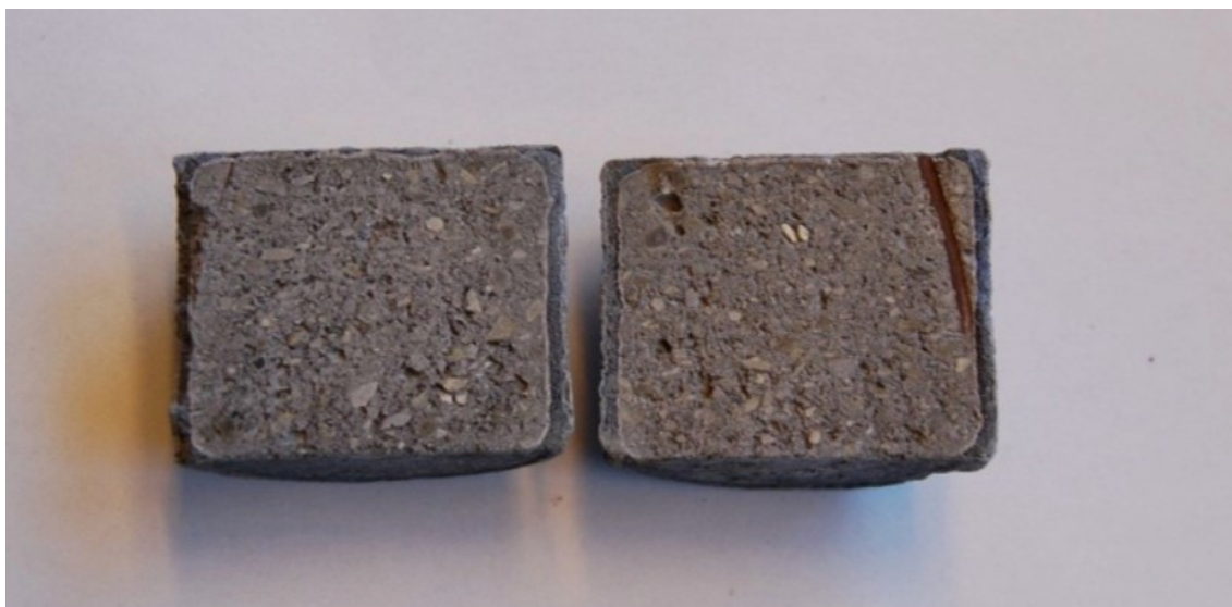
Figure 6. Cross-section of sample after Test 5, where Alubar 1100 was embedded in \text{AlF}_3 at 900^\circ\text{C} for 3 hours, without electrolysis.
