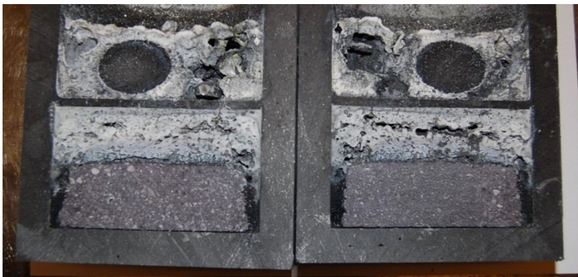
Figure 4. Cross-section of crucible after Test 3 with \text{Al}_2\text{O}_3 as bedding material.
