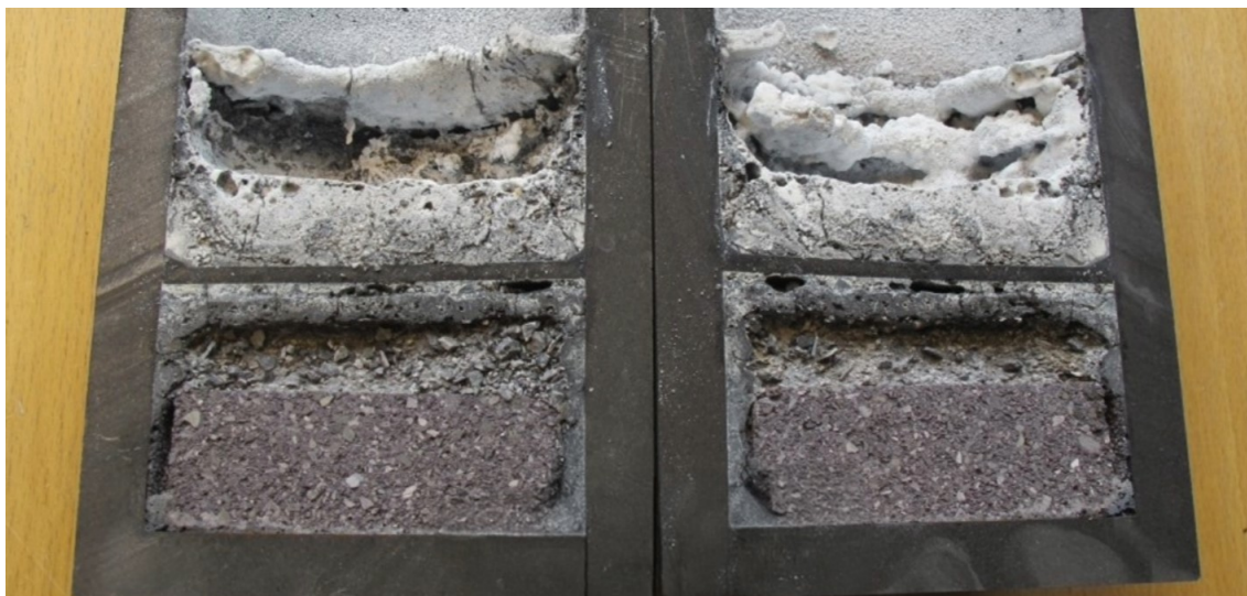
Figure 9. Cross-section of crucible after Test 8 with Clayburn Dri-Barrier Mix as bedding material.
