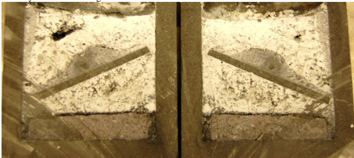
Figure 2. Cross-section of crucible after Test 1 with AlF 3 as bedding material.
